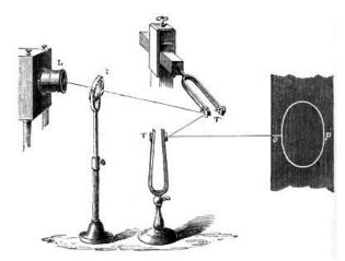
Schematic drawing of Lissajous' machine
